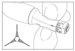
put the propeller's blade in feathering position.
