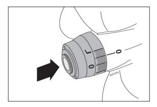
release the ogival nose. make sure that the reference line «0» matches the desire notch.
