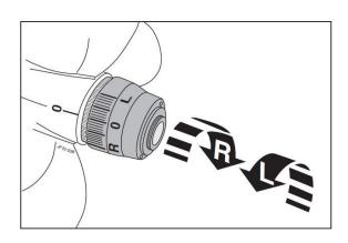
Turn the ogival nose towards the «R» or «L» side depending on the type of engine (rightway or leftway) and reach the notch of the desired pitch.
